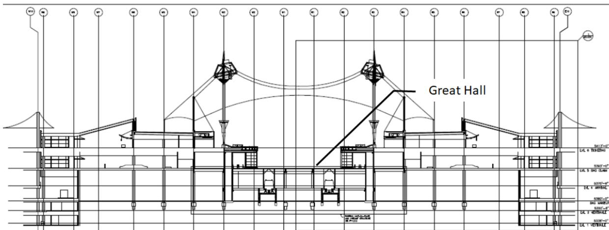
**Figure 3. Cross-section through main terminal complex**
