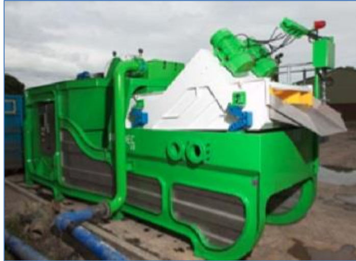
Figure 2-11 Anaergia’s Hydrocyclone for Organics Polishing
