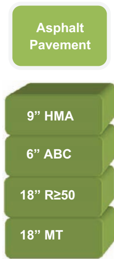
Figure 8.3: US 36 Phase 2 Asphalt Pavement Structure
