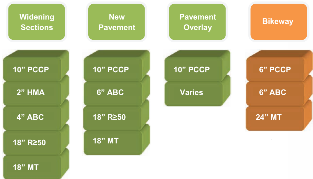
Figure 8.2: US 36 Phase 2 Concrete Pavement Structures
